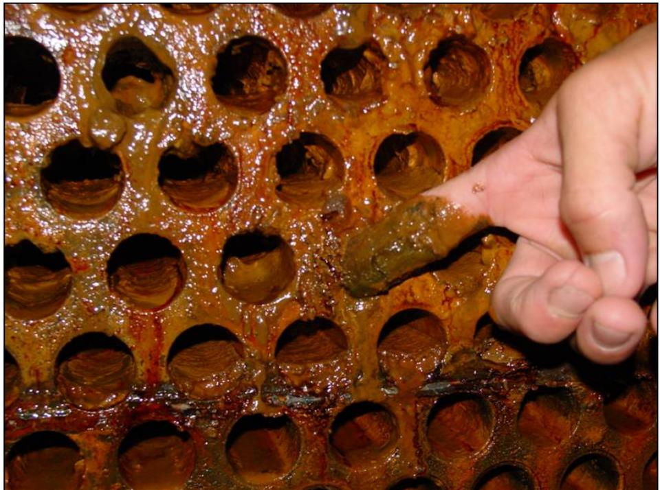
*Heavy biofilm fouling of condenser tubes. Biofilm is more resistant to heat transfer than scale and promotes under-deposit corrosion.*
