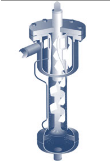
Centrifugal separators provide an alternative for solids removal in cooling tower systems. Cooling system blowdown can be used to purge solids from the bottom of the separator, minimizing or eliminating unnecessary water loss.
