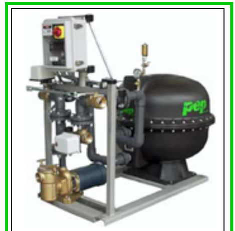
Granular media filters like the one shown here are good options for cooling tower systems with heavy particulate loading. The unit automatically backwashes a preset pressure differential when the media bed becomes fouled.
