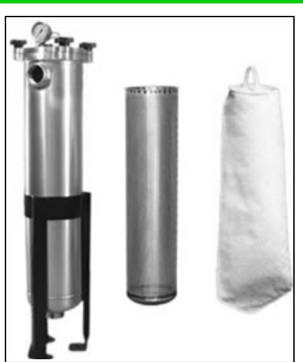
A typical bag filter. This unit has a filter basket that holds the filter bag. Bag filters provide an alternative to cartridge filters. Most filter bags can be cleaned and re-used several times, saving on replacement costs.
