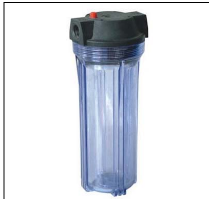
A simple single cartridge housing like this one is all many small closed loops require for good filtration. A unit like this can provide good results in loops up to 5000 gallons or greater total water volume if the loop was adequately cleaned and a good chemical treatment program is in place.
